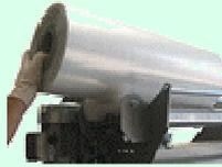
**Automatic end of spool system** is a safety system that stops the film entering the rollers when the spool is finished, thereby avoiding possible damage and prolonged system downtime.
