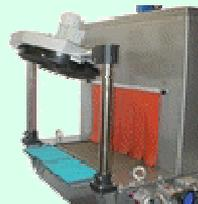
**Pneumatic product pressing unit** for unstable packages, with adjustable height, holds the package in position before the welding bar descends
